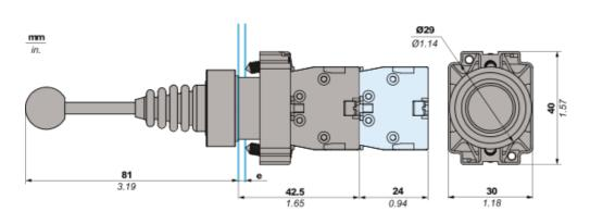
e: clamping thickness 1 to 6 mm / 0.04 to 0.24 in.
