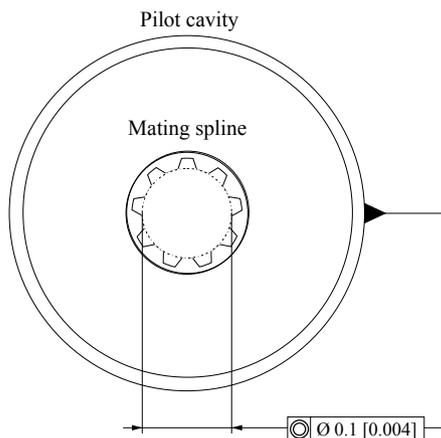
Use **plug-in drives** if the concentricity between the mating spline and pilot diameter is within 0.1 mm [0.004 in]. Lubricate the drive by flooding it with oil. A 3-piece coupling minimizes radial or thrust shaft loads.
