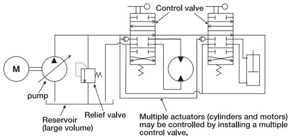
1. In the open circuit, oil is drawn by the pump from the reservoir, and the returning oil from the actuator is flown to the reservoir.
