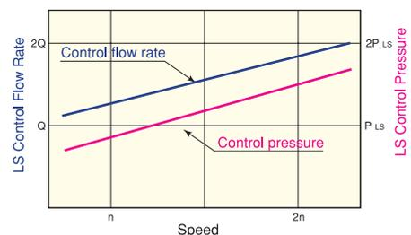
※ It is possible to control the flow rate almost proportional to the pump rotating speed.
