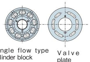
Single flow type cylinder block
