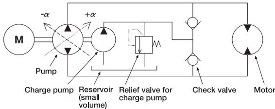
1. The closed hydraulic circuit is constructed with an actuator (motor) and a pump.
