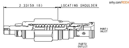
Direct-acting relief cartridges are normally closed, pressure-limiting valves used to protect hydraulic components from pressure transients. When the pressure at the inlet (port 1) reaches the valve setting, the valve starts to open to tank (port 2), throttling flow to limit the pressure rise. These valves are smooth and quiet, essentially zero leak,
