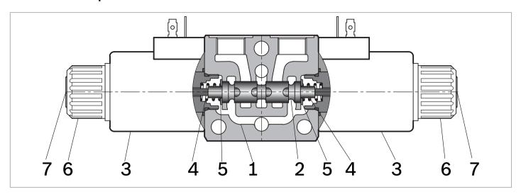
The sandwich plate design directional valve elements L8080... are compact direct operated proportional solenoid valves which control the start, the stop, the direction and the quantity of the oil flow. These elements basically consist of a stackable housing (1) with a control spool (2), one or two solenoids (3), and one or two return springs (4).
