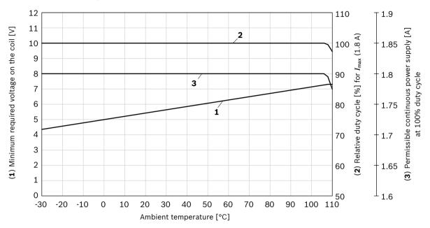
**▼ 24 bar control pressure, 12 V** ( $R_{\text{nom}}$  = 2.4  $\Omega$ ;  $I_{\text{max}}$  = 2.2 A)
