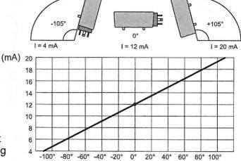
Attention: the input resistance of the used instrument (for the measurement) must have a value that allows to the sensor to supply the maximum current.
