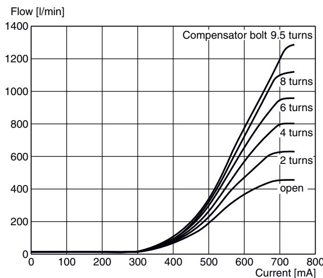
The diagram shows the control curves for spool "81-10" with different compensator settings.
