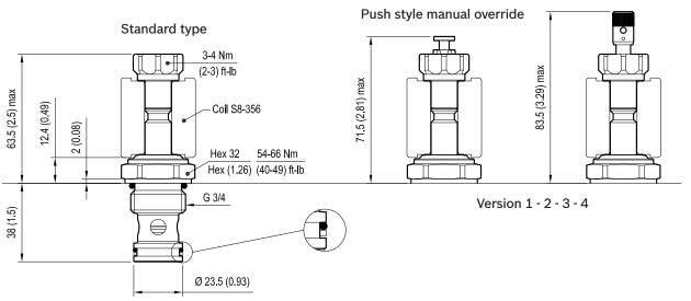
Version 2: Solenoid operated valve, poppet 2-way normally open Version 3: Solenoid operated valve, poppet 2-way double lock normally open
