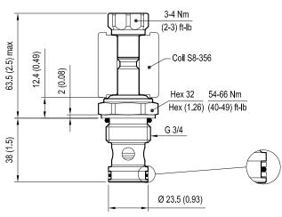
Version 4: Solenoid operated valve, poppet 2-way normally open
