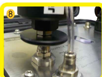
Check for flush fitting
