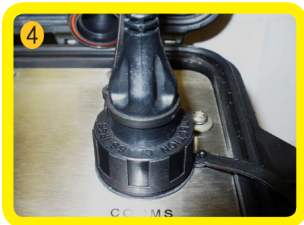
4 Ensure the RJ45 is fully screwed down. Do not over-tighten.
