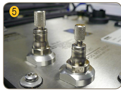
To avoid fluid leaking after use, fit the blanking plugs (ACC6NN033)
