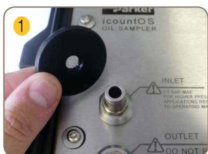
Orientate PRV removal tool
