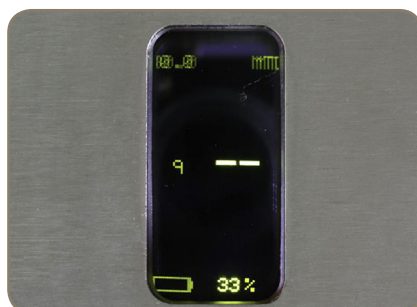
...and the alarm limit setting: 9.
