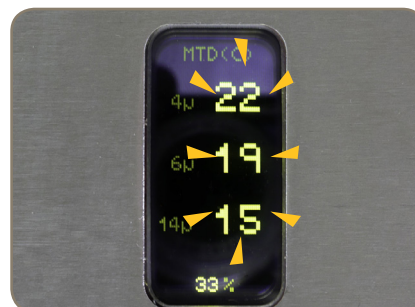
The contamination level numbers flash if alarm levels have been reached (see 'Configuration page – ISO', page 26).
