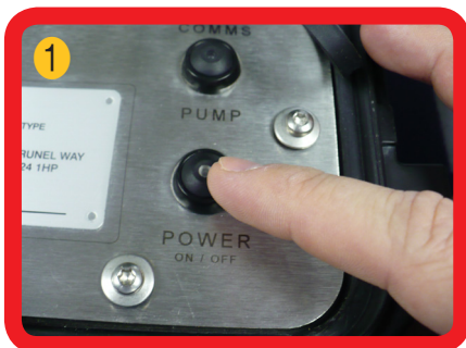
Switch off the inlet pressure and the POWER switch before removing the hoses. The power light may still flash if connected to a mains supply.
