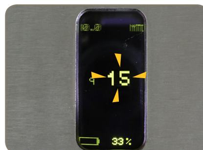
The contamination level number flashes if the alarm level has been reached (see 'Configuration page – NAS', page 26).
