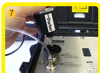
Press PRV firmly into INLET port
