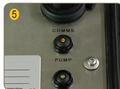
Pump on, test starts
