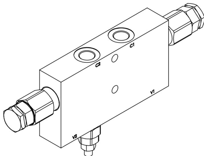
MAX FLOW: 40 lpm (10,57 US GPM)
