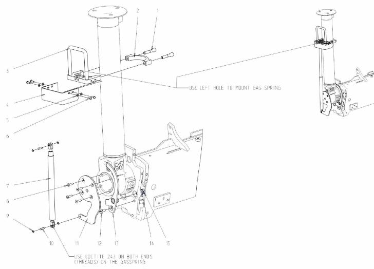
THE GAS SPRING MUST BE MOUNTED WITH THE LEG IN 170° NOTE MOUNTING DIRECTION OF GAS SPRING
