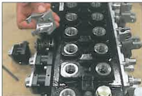
16. Tighten the spring bolt to 10-15 Nm with the 17mm socket wrench before taking away the spring holder and mounting the spring cover.
