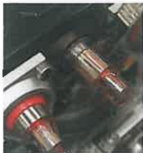
15. Place grease around the spool on both sides of the seal and on the console. Then mount the console and the lever link.
