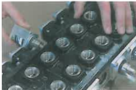
13. Gently push the spool into the valve.
