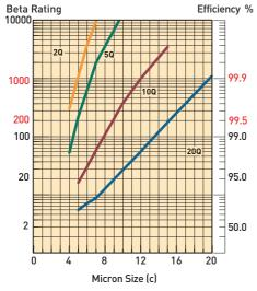
Notes: Multipass test run @ 80 gpm to 50 psid terminal - 5 mg/I BUGL.
