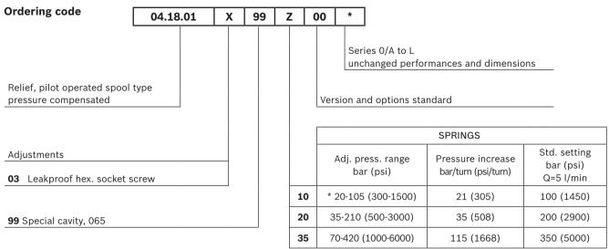
Minimum pressure setting intended with Q=5 I/min. (1.3 gpm)
