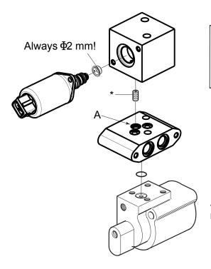
Solenoid PS25 for valve HV08 always assembled with restrictor  $\Phi$ 2.0 mm! (PS25 as spare part is always delivered with restrictor  $\Phi$ 2.0 mm.)
