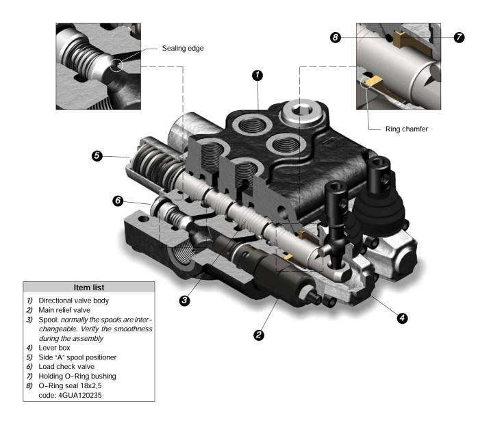
NOTE - All articulated parts inside cap, lever box and mechanical joystick are lubricated with synthetic base grease grade NLGI2
