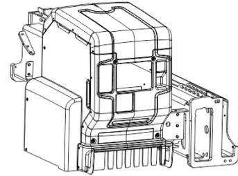
Remove cover when the crane is equipped with a display.
