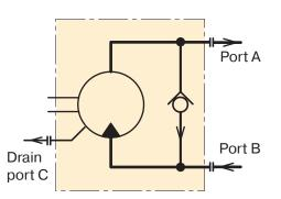
Hydraulic schematic, the motor is shown with make-up valve; shaft rotation 'R' (MUVR)
