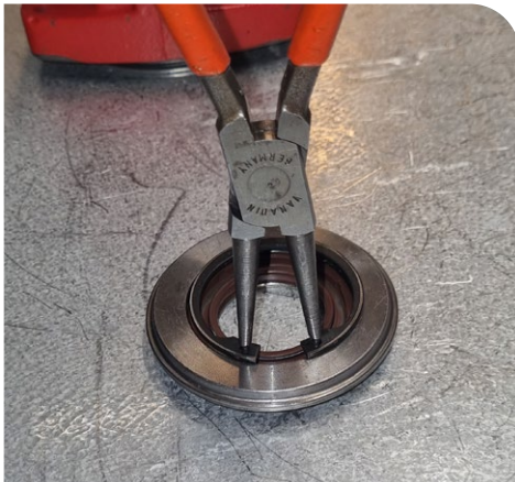
11. Disassemble the retaining ring (item 238)
