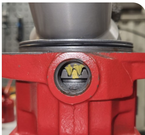
31. Install the O-ring (item 221) Included in seal kit
