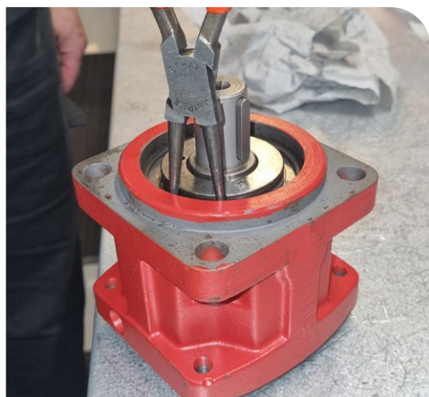
30. Install the retaining ring (item 237) Included in seal kit Tips! Tap with mandrel and hammer to secure retaining ring is correct assembled.
