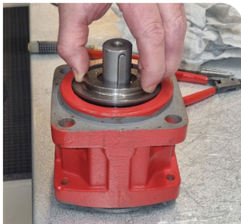
29. Install the seal carrier (item 231)
