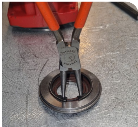
28. Assemble the retaining ring (item 238)
