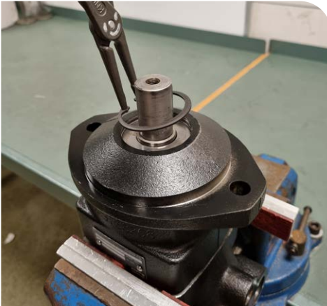
3. Disassemble the retaining ring.
