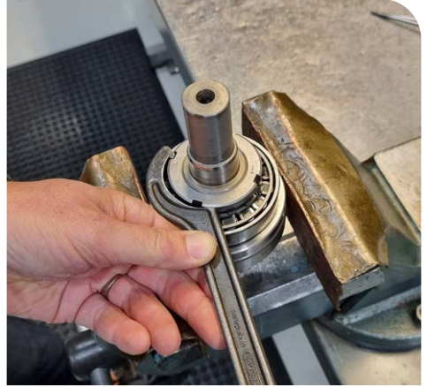
14. Untighten the round nut and remove locker rings.
