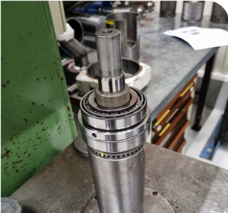
15. Place the shaft package on a tube so it's standing on the ring gear. Press the shaft off the bearings. Use some soft material when the shaft fall out.
