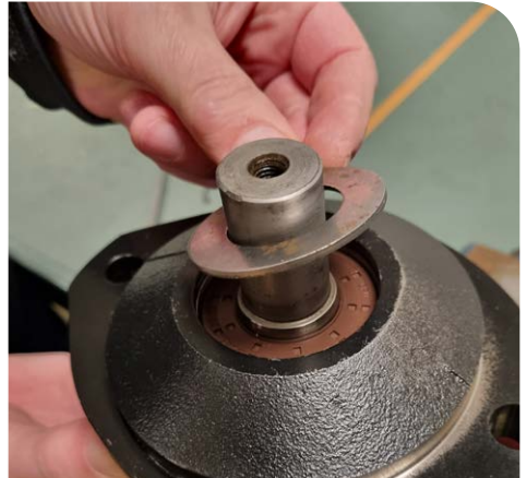
4. Remove the back up ring.
