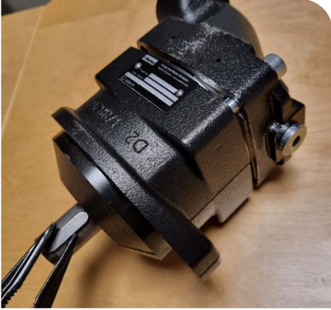
1. Remove the key with a plier.
