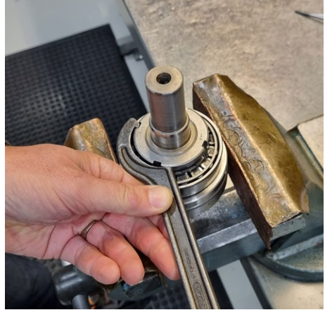
14. Untighten the round nut and remove locker rings.
