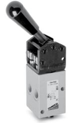
The manual valves Series 3 (G1/8) and Series 4 (G1/4), 3/2 - 5/2-way and 5/3-way, are available with devices designed to satisfy different needs. The 3/2-way valves Series 3 and 4 are normally closed when 1 is the inlet; they can also be normally open when 3 is the inlet.
