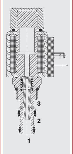
When de-energized, the valve allows flow from port 1 to 2 or from port 2 to 1, while blocking flow at port 3. When energized, the valve allows flow from port 3 to 2 or from port 2 to 3, while blocking flow at port 1.
