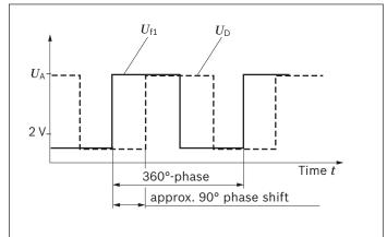
Frequency signal and direction of rotation signal can be evaluated in the measurement range from 0.1 Hz to 20 kHz.
