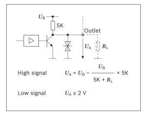
The output circuitry for the rotational speed signal and the direction of rotation signal are identical.
