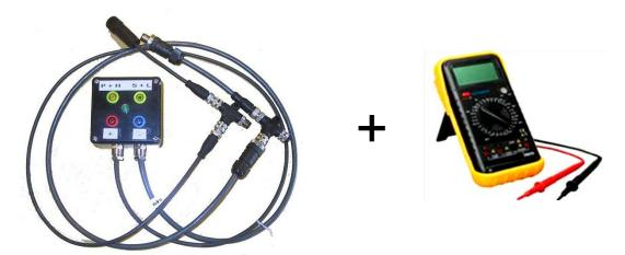
Dismount the M8/M12 plug from the sensor/the module that you wish to diagnose and then place the Diagnostic Box between the plug and sensor/CAN bus module by means of the cable that comes with the box.
