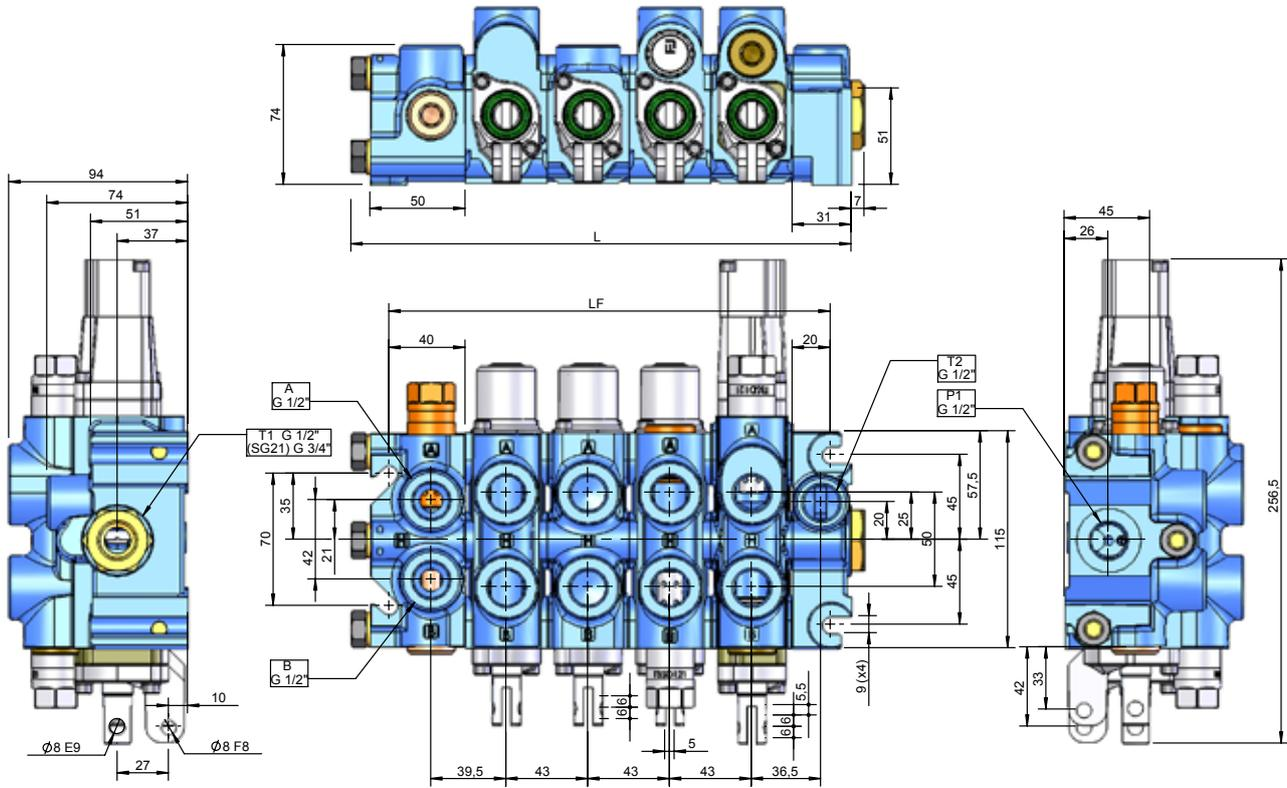
**I01A** has two pump ports and one tank port.
