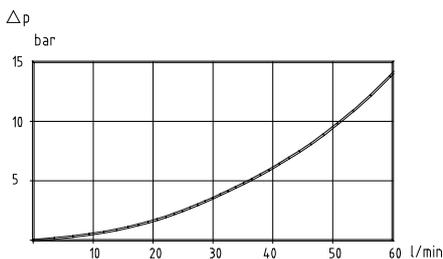
Pressure drop, P1 - T4, inlet I01E, unloaded
