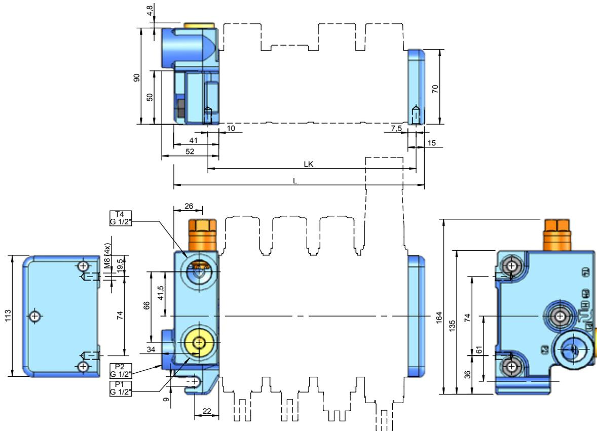
**I02C** has two pump ports and one tank port. The main relief valve cavity is on the A-side.
