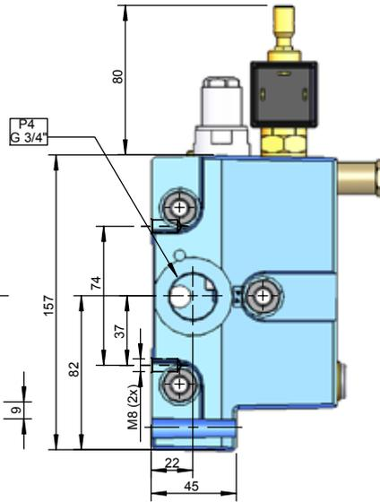
**I06Q** has the same functions as I02Q but with an added special check valve FSB3 in the signal gallery to damp the unloading function of the flow control valve FKA. I06Q also provides an additional pump port.
