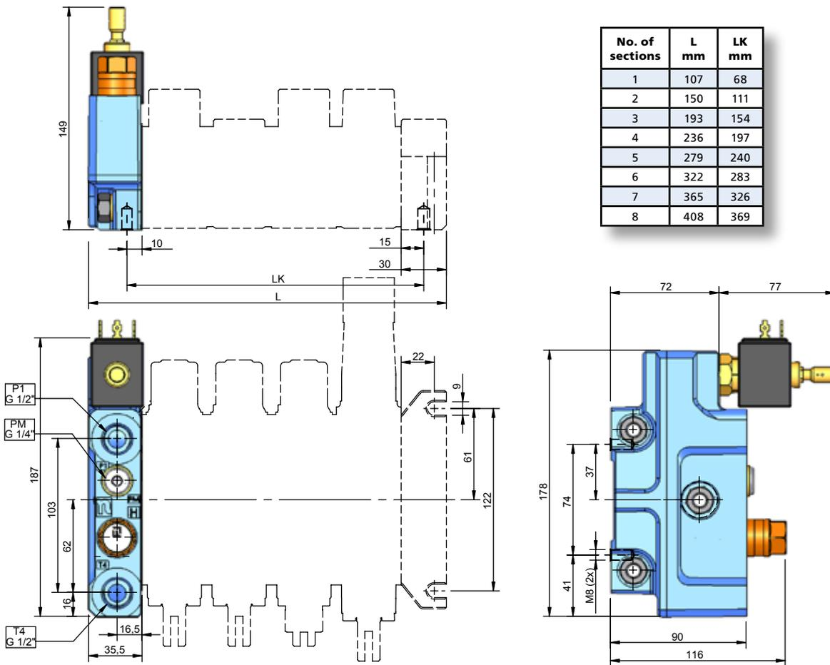
**I01E** has one pump port and one tank port, both facing upwards. The main relief cavity is facing upwards. Main relief options: TBD160 up to 300 bar and TBS400 up to 350 bar.
