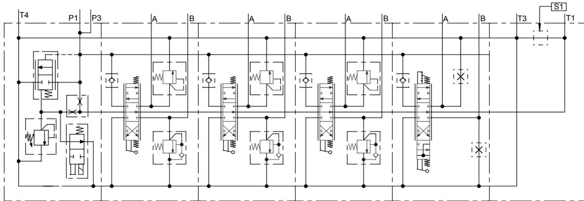
Hydraulic circuit diagram for a four sectional RS 210 valve. It is fitted with a Q-inlet with electrical unloading. The first three sections contain 3-positions spools for double acting functions and port relief and anticavitation valves. The fourth section contains a 4-position spool for double acting functions with float position in position 4. The outlet gives possibility for high pressure carry-over (if S1 is plugged).
