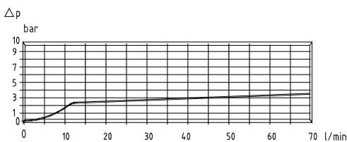
Pressure drop P1 - T4, inlet I02Q/I06Q, unloaded
