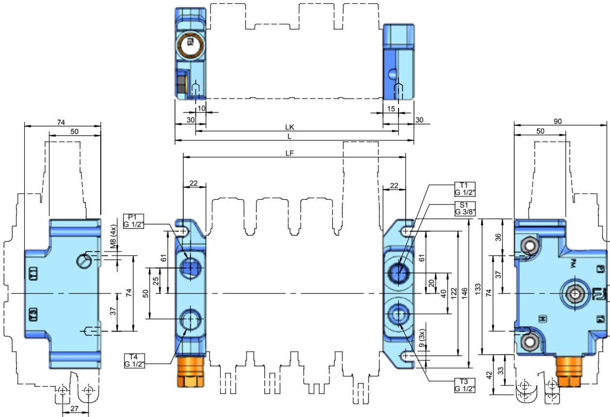
**I06B** has one pump port and one tank port, both facing upwards. The main relief cavity is on the B-side.
