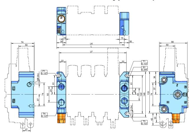
**IO6B** has one pump port and one tank port, both facing upwards. The main relief cavity is on the B-side.
