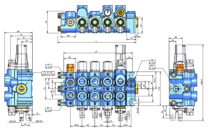
**I01A** has two pump ports and one tank port.
