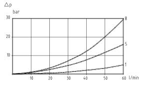
Pressure drop, P1 - T1/T3, inlet I02C, outlet U01B
