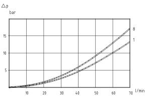
Pressure drop A/B - T, inlet I06B, outlet U01B
