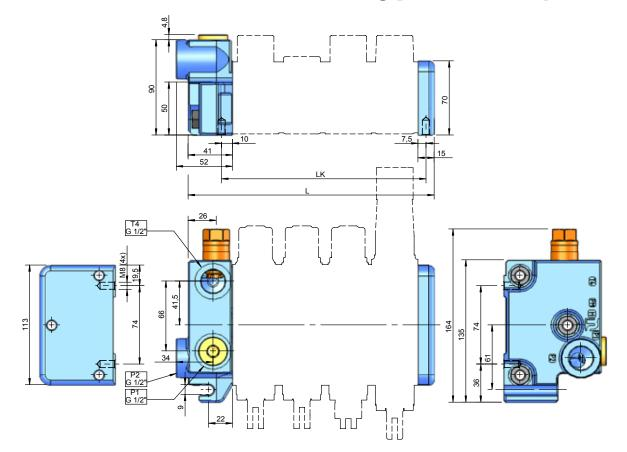
**IO2C** has two pump ports and one tank port. The main relief valve cavity is on the A-side.
