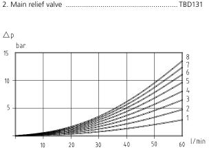
Pressure drop, P1 - T1, inlet I06B, outlet U01B
