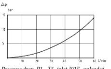
Pressure drop, P1 - T4, inlet I01E, unloaded
