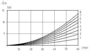
Pressure drop, P1 - T4, inlet i02C, outlet U01C
