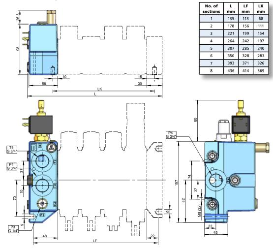
**IO6Q** has the same functions as IO2Q but with an added special check valve FSB3 in the signal gallery to damp the unloading function of the flow control valve FKA. IO6Q also provides an additional pump port.
