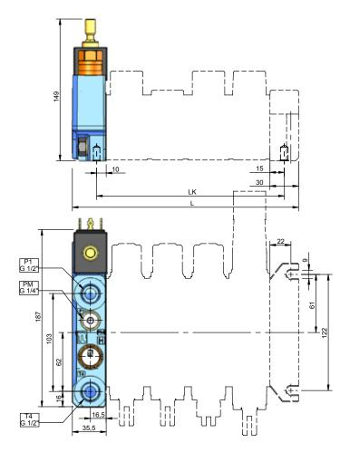
**IO1E** has one pump port and one tank port, both facing upwards. The main relief cavity is facing upwards. Main relief options: TBD160 up to 300 bar and TBS400 up to 350 bar.
