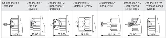
In case of solenoid malfunction or power failure, the spool of the valve can be shifted by manual override as long as the pressure in port T does not exceed 25 bar (363 PSI). For alternative manual overrides contact our technical support.
