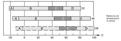
E.g. Hydraulic oil 32: The designation "32" denotes the viscosity is 32 cSt at 40 °C. Lowest start temperature will be -23 °C and highest working temperature 82 °C. Ideal working temperature is 35 - 55 °C.
