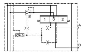
Without adjustable LSA/B pressure limiting valves With non-damp pressure compensator valve With facilities for shock valves A/B
