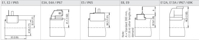
The specified IP rating applies only in the case of correctly connected connectors (male + female) with the corresponding IP rating.
