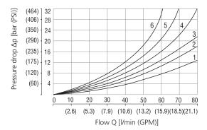
P-A P-B A-T B-T P-T P-A P-B A-T B-T P-T Spool symbol Z11,L21,B11,R11 P51 2 2 3 3 3 R21,X11,N11,J15 Y51 C51 2 6 H11 3 4 Z71 3 Z81 3 Z91 3 3 Y41 Z21,Z51,H51 C41 R31 3 2 3 4 F51 4 5 3 K11 3
