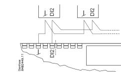
The following controllers can be connected up in this way: EKC 202D, EKC 202D1, AK-CC 210 (But max. 15 controllers)
